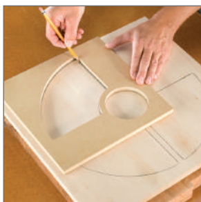
Trace the templates onto the bowl blank.
